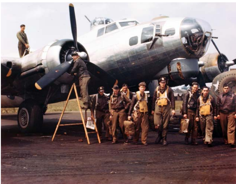
Back from bombing an airdrome near Bordeaux, the Sam Whitehead (center front) combat crew of the Boeing B-17 Patsy Ann heads for interrogation while ground crewmen make routine checks on oil and engine. Man on wing holds nozzle of oil hose which runs up from tank truck. On the ladder, a mechanic inspects the inside ring cowlings of the right inboard engine for possible flak damage or malfunction. 534 th Bomb Squadron, 381 st Bomb Group, Ridgewell, England. Image 8393a, NARA 2016 Folder, EAAWP.
